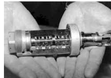
The B-737's main rudder power control unit (right) contains several subassemblies, including a servo valve (cut open for display purposes, left) that directs hydraulic fluid to the rudder actuators.
